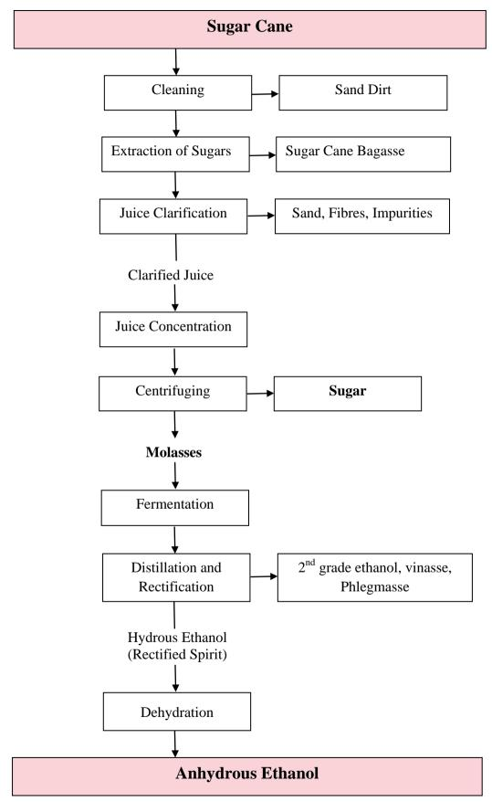
**Annexure 1: Flow Diagram of the Ethanol Production Process**
